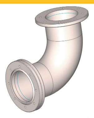
CMM readings are imported into computer-aided design (CAD) software to show the impact of alternative flange re-facing scenarios. Finite element analysis points to high-stress and low-stress areas in the pipe connections. The Dimensional Engineering team tests and tweaks the flange re-facing plane in the coordinate system until determining how to stop the leak with the least amount of bending and pulling on mating flanges and gaskets.
